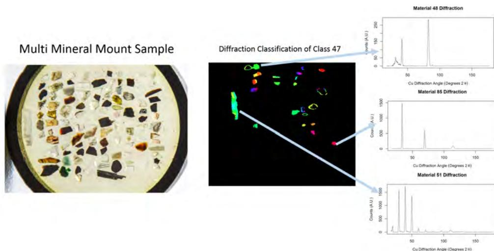
**Figure 1:** (Left) A photograph approximately 100 minerals in a flat polished epoxy mount. (Right) A mask of class 47, as identified using an SOM on the XRF data, then again on the XRD data to identify the materials present. The diffraction patterns from some of those materials are shown on the right.
