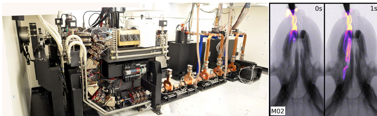
Figure 1: Left: Photograph of the Lyncean Compact Light Source. Right: Example of a dynamic in vivo imaging application, showing delivery of liquid instillations to the nose of a mouse [1].
